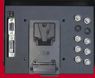
LCD- 703HDV Unit with "V" lock mount for IDX batteries
